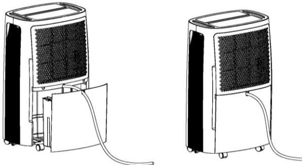
**Note:** Water pipe cannot be too long (usually 0.6m or 1m), the height cannot surpass the height of drainage mouth, or there will be water leakage.
